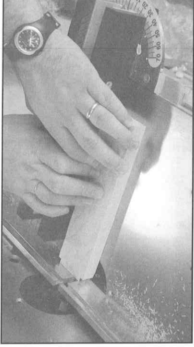
Fig. 14-1: Making top cheek cut. Feed workpiece from right-to left using miter gauge. Inset shows cut.
