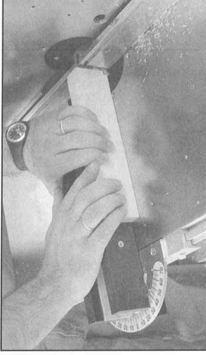
Fig. 14-1: Making top cheek cut. Feed workpiece from right-to left using miter gauge. Inset shows cut.
